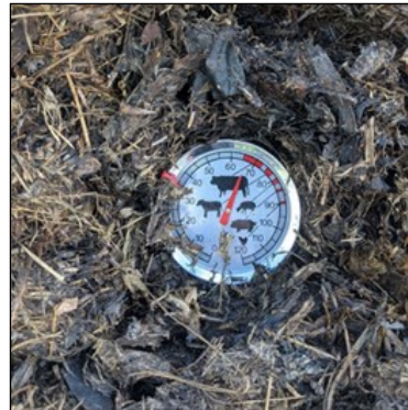
Days 1-4. Stable temperature of 65°C over the next 4 days. This is a meat thermometer so its probe is fairly short. Dedicated compost thermometers are available.
