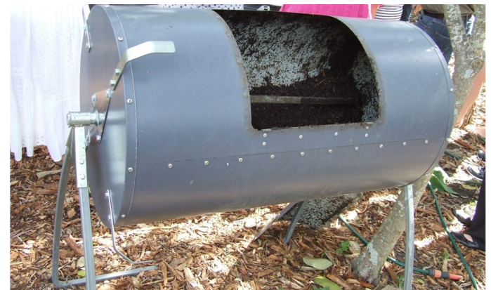
Cylindrical compost drum rotates to mix the food scraps and other materials which then go in the first bin.
