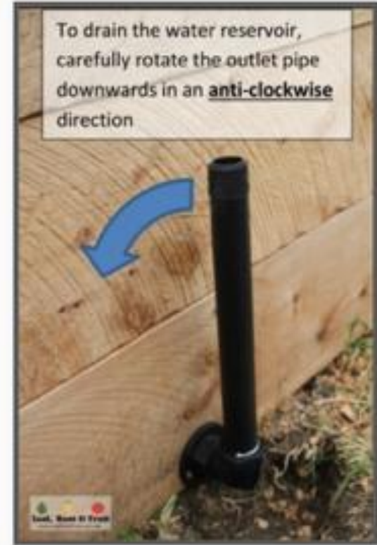
A wicking bed water outlet, water level indicator and reservoir drainage valve all in one.
